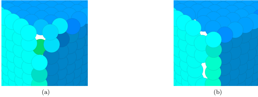
Figure 4: This figure shows the effect of the proposed constraint-based vertex position update scheme: Figure (a) represents the point set reconstructed by using Equation (14) not only for flat regions but also for feature points. Figure (b) represents the result obtained by the proposed scheme, where flat regions follow Equation (14), edges are reconstructed using Equation (13) and corner positions are updated using Equation (11). Note how the corner itself is not recovered in (a), but is recovered in (b).
